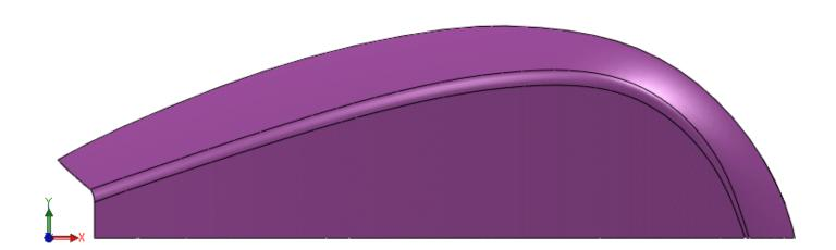
2. Create a curvature continuous fillet surface connecting the top and side surfaces.
